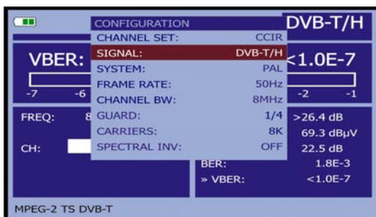
Figure 20.- Screen of measurement configuration (COFDM signals).
