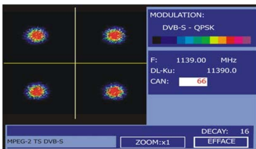
Figure 49.- Diagramme de constellation. Signal DVB-S (QPSK).
