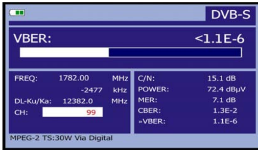
Figure 40.- DVB-S (QPSK) signals VBER measurement screen.
