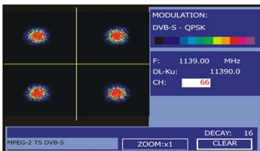
Figure 49.- Constellation Diagram. DVB-S (QPSK) signal.
