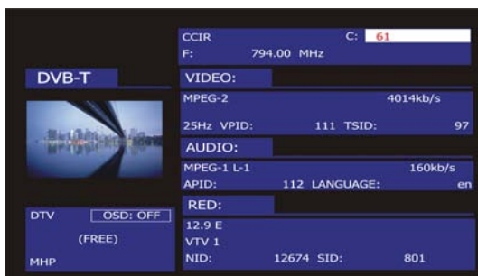
Figure 70.- Digital channel monitoring.
