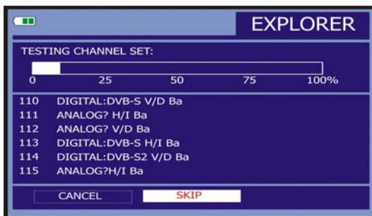
Figure 18.- Spectrum exploration screen.
